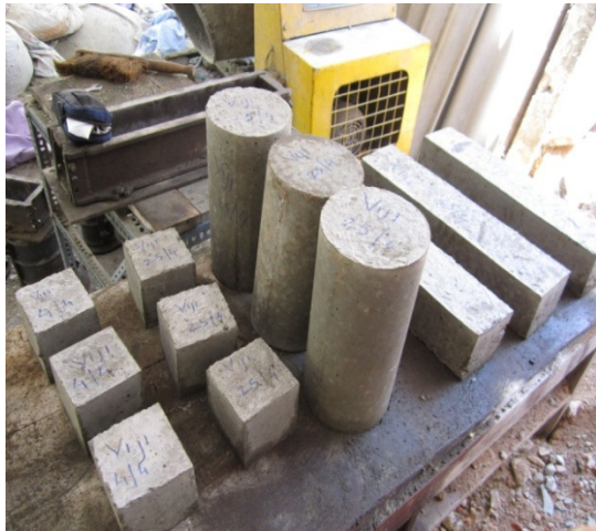
Fig.5 Casting of specimen
